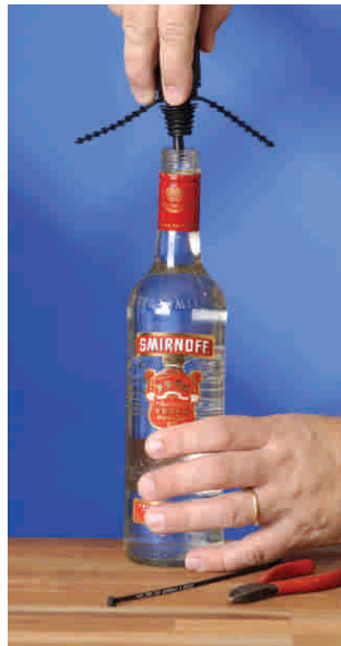
Spouts are easily mounted with a decompression tool. Sealing ties are fixed and new bottles are ready for inventory.
