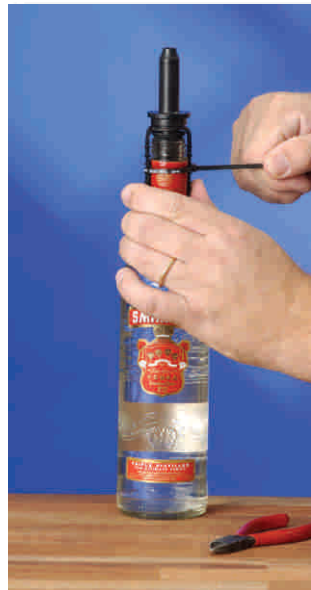
Spouts are easily mounted with a decompression tool. Sealing ties are fixed and new bottles are ready for inventory.
